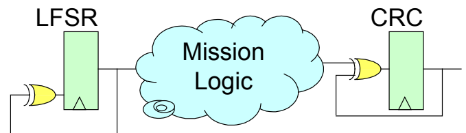
Figure 3. Signature analysis method replaces stimulation ROM with a test pattern generator, and the compare ROM with a sequential signature check circuit.
